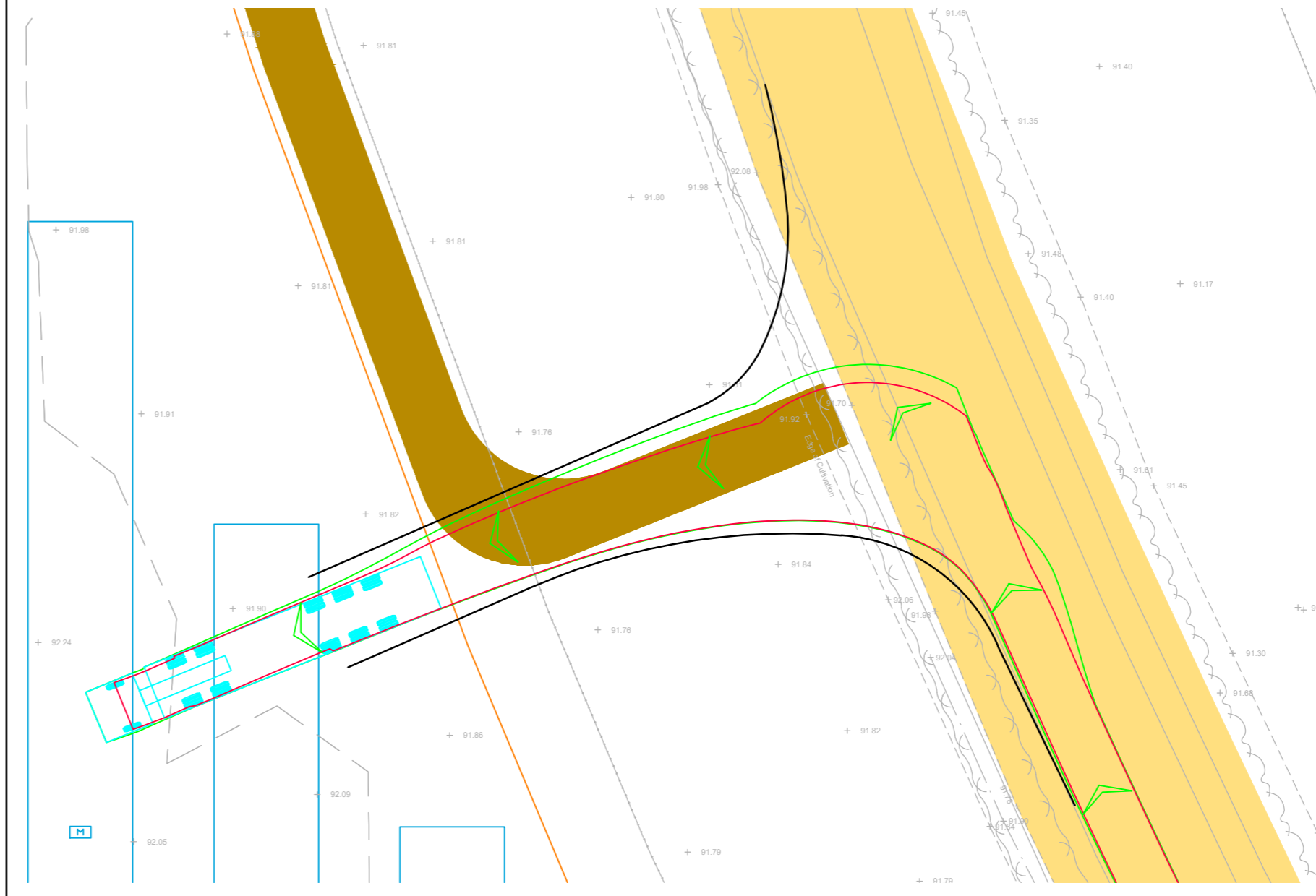
Swept Path Analysis A 16.5m Articulated HGV Entering
