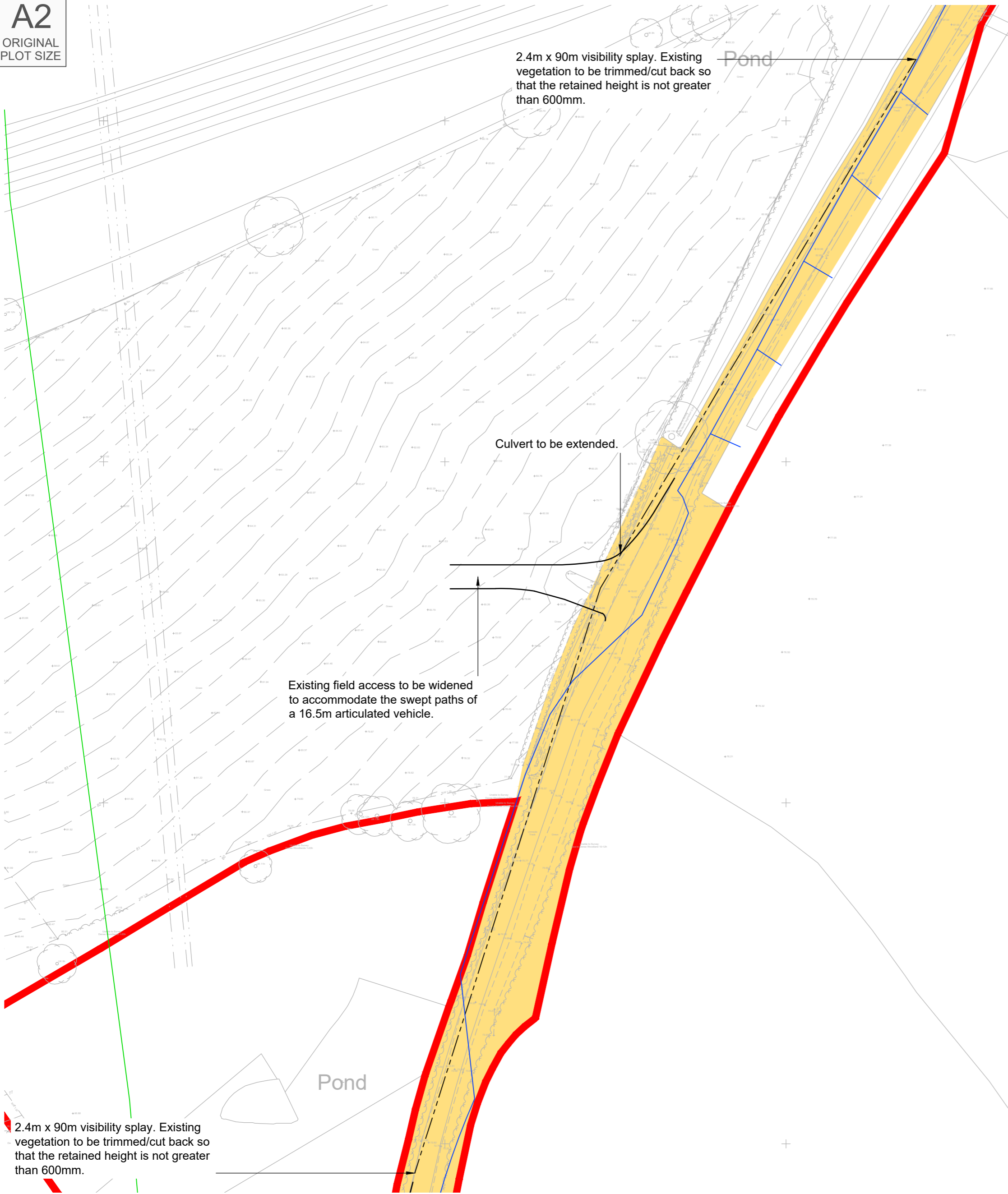
Proposed Site Access Arrangement Scale 1:500
